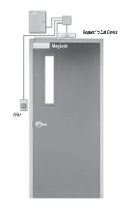
Note: Securitron's UL294 certification indicates that when the EEB is used with the XMS Motion Sensor, it meets the NFPA Life Safety Code 101 requirements for exit of access-controlled egress doors.
