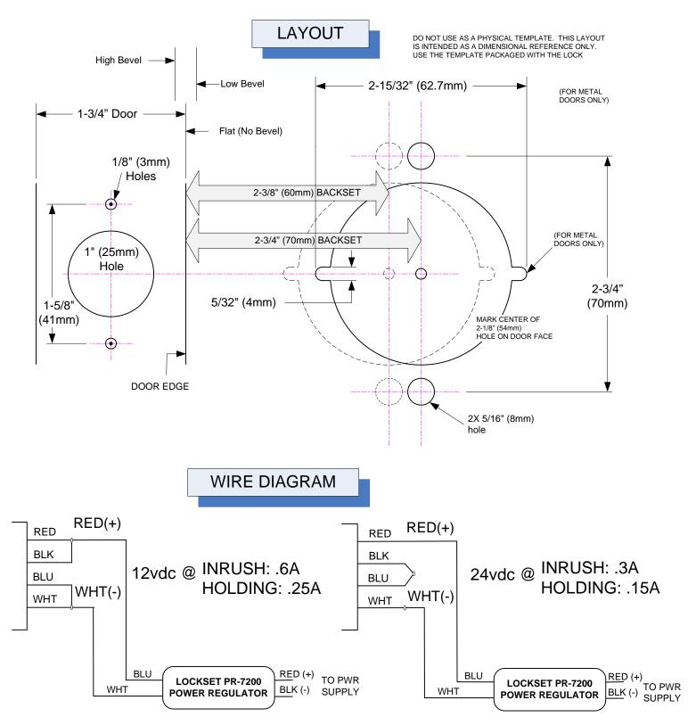
Use of the PR-7200 limits the power consumption, reduces operating temperature, and suppresses inductive kickback.
