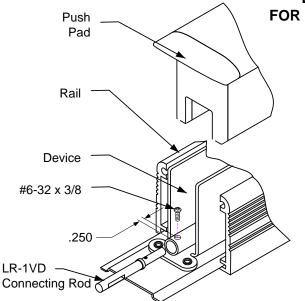
When retrofitting to existing vertical rod devices, adjustment of the rods are required for proper assembly of the LR100VDK Kit. Please see the SDC website (www.sdcsecurity.com) for installation tips and photographs of installing.
