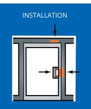
SDC Spacesaver<sup>®</sup> locks may be mounted in the frame header, side jamb or door lock stile.
