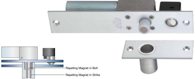
The **FS23M** dual failsafe feature is available only from SDC. Conventional failsafe locking bolts rely solely on a spring to retract the bolt while the FS23M bolt will unlock with or without the assistance of the spring. This is the only electric bolt lock listed by the California State Fire Marshal for locking of perimeter entrance and emergency exit doors after-hours.
