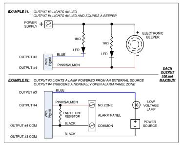
Fig. 5 Using Solid State Outputs
