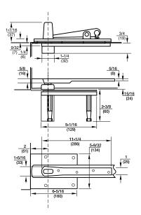
Center hung pivots are door hanging means only. To close doors, see floor closer sections of the catalogs.
