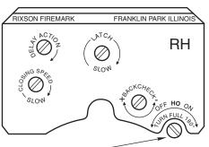
Do not use Backcheck as deadstop. This is an intensity valve not speed control.
