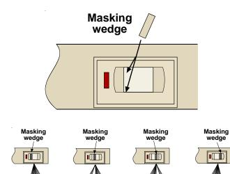
Insert a masking wedge by placing the bottom peg in first. Then press on the center of the wedge until it snaps into place.
