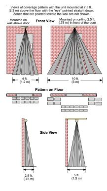
The higher the unit is mounted, the larger the coverage area. Do not mount the DS160/161 more than 15 ft. (4.6 m) above the floor.
