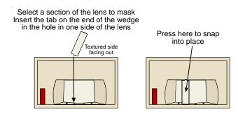
Remove a wedge by placing the tip of a small screwdriver behind the wedge and prying it up. Do not scratch the lens when removing the wedge.
