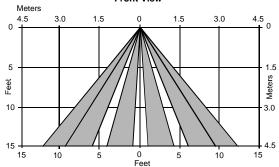
Figure J - Standard Patterns for a Wall Mounted Unit
