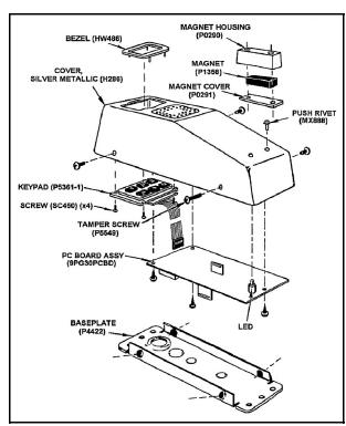
Fig. 4. Exploded view with part numbers.
