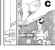
Remove lock cover. A. Remove spring from Locking Piece Assembly and lift Assembly out.
