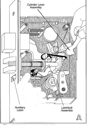
A Marionalian Auxiliary Washer j, IF REVERSE HANDING IS REQUIRED: Remove lock cover. A. Lift out Cylinder Lever Assembly. Pull back
