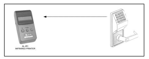
Scenario 3 Use the AL-IR1 Infrared printer to print your lock's audit trail (event log), User Code list, clock settings and software version. No cable required.
