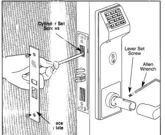
**INSTALLING CYLINDER AND LEVER** A. Thread Cylinder through Outside Assembly and tighten up as far as possible. Make sure keyway is at the bottom of cylinder. C. Tighten the Cylinder Set Screw nearest the cylinder.
