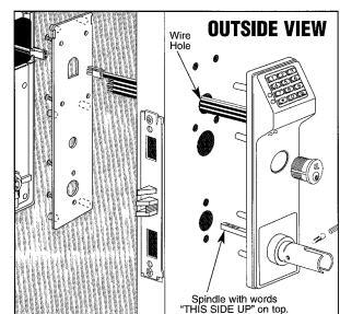
INSTALLING LOCK AND OUTSIDE TRIM ASSEMBLY Insert lock into cavity and fasten with 2 screws.
