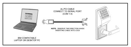
If your computer does not have a serial COM port (DB-9 male) available, you can plug your AL-PCI2 cable into a special USB to RS-232 cable. Order part PCI-USB for the USB to RS-232 cable only, or ALPCI2-U for both the USB to RS-232 cable and an AL-PCI2 cable).
