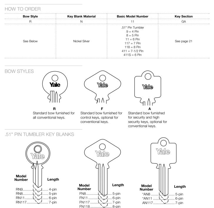
\*Standard keybow for high security key blanks, letter of authorization required. Side cuts are factory machined.
