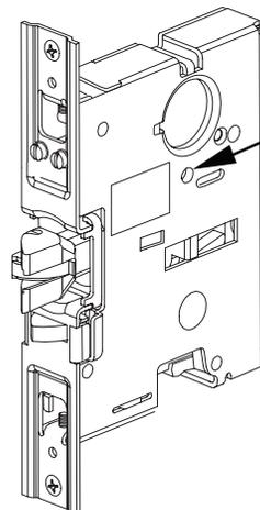
For mortise device applications, NL screw located on side of 7500 mortise lock remains as shipped for NL operation. As shipped position is when NL screw is turned out counterclockwise. For any questions, contact technical support.
