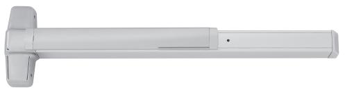
9848/9948 Concealed vertical rod device for use on single or double metal doors, UL listed for panic exit hardware. Covers stock hollow metal doors with 86 or 161 cutouts. Devices are ANSI A156.3 – 2008 Grade 1. The 9848 device has a smooth mechanism case and the 9948 device has a grooved case. The concealed vertical rod device is non-handed except when the following device options are used:SD (special dogging), or SS (signal switch). See opposite page for available outside trim and functions.
