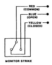
NOTE: SWITCH POSITION SHOWN WITH TRIPPER DEPRESSED, IE: LATCH BOLT IN STRIKE.
