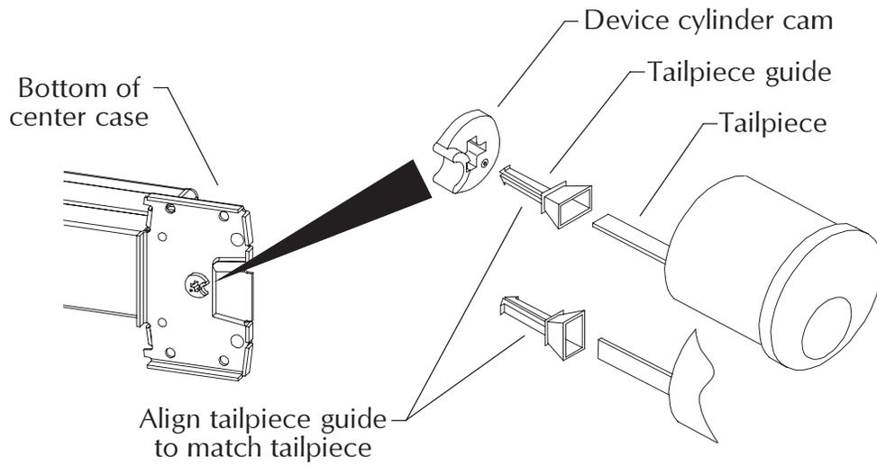
3.2. Install device to door at center case.
