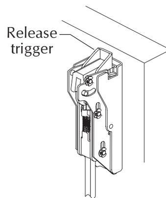
**11 Install and adjust bottom rod.**
