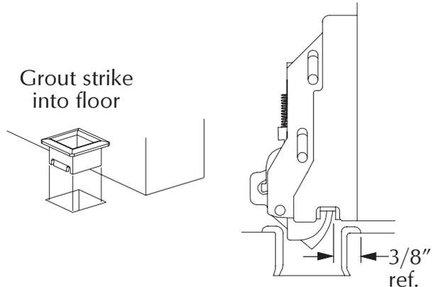
**7 If door height is less than 84", cut top rod. (Uncut top rod is about 38-3/4" overall.)**
