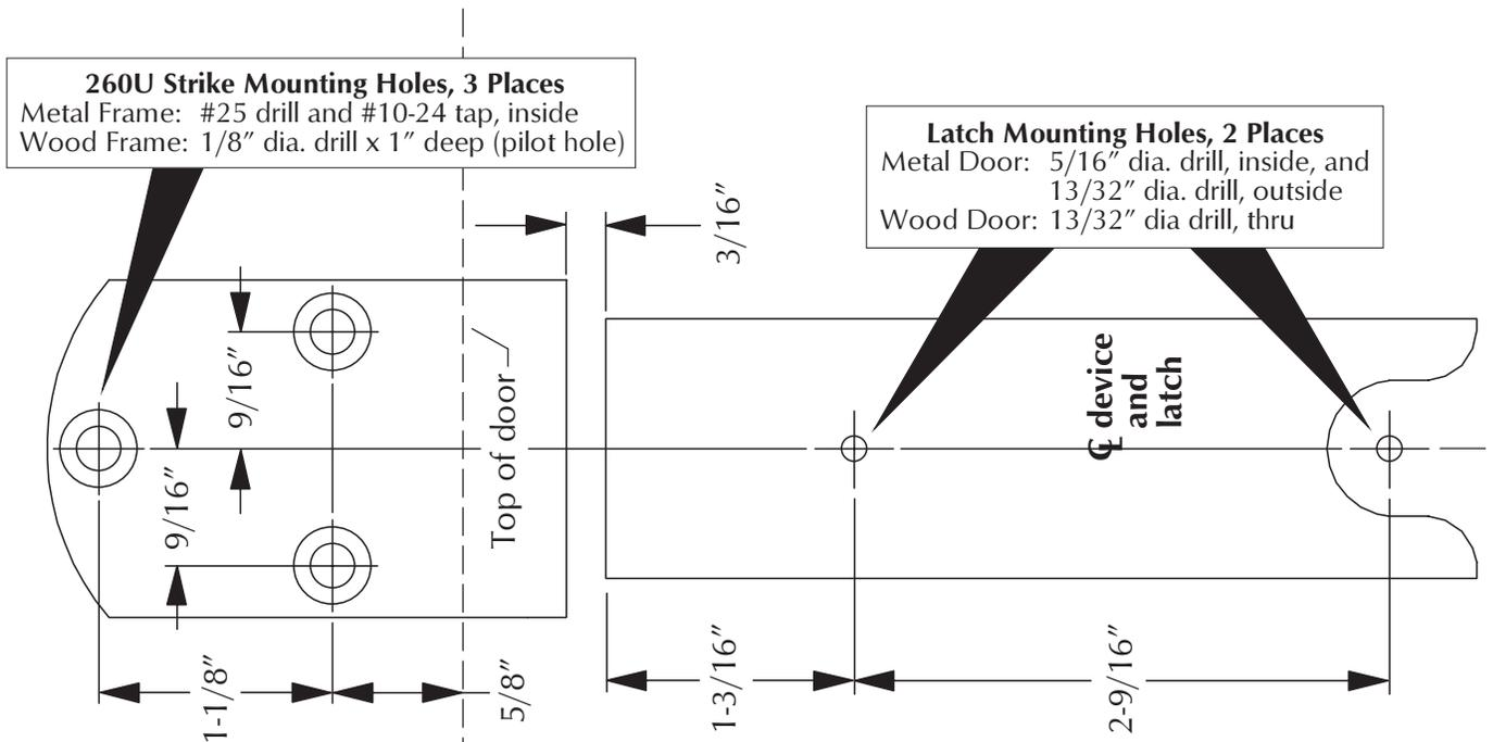
Refer to Step #2 when using these templates. Templates to scale.
