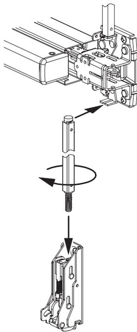
**Adjust (screw rod into or out of latch)**
