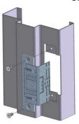
**INSTALL THE** 478-ANSI-ITL INTO THE THE FRAME **USING THE SUPPLIED MOUNTING SCREWS.**
