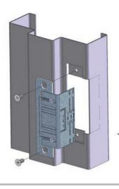
**REMOVE THE TEMPLATE FROM** THE FRAME, **EXPOSING THE SCRIBED GUIDE** LINES.
