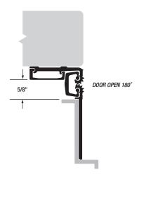
**MATERIAL:** Extruded 6063 T6 aluminum alloy with self-lubricating polyester thrust bearings.
