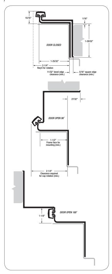
**MATERIAL:** Extruded 6063 T6 aluminum alloy with self-lubricating polyester thrust bearings.
