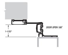
**MATERIAL:** Extruded 6063 T6 aluminum alloy with selflubricating polyester thrust bearings.
