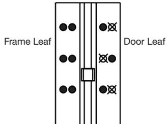
6. Mark (or centerpunch) holes. If using SDTF screws, go to Step 7. If using TF or wood screws, drill holes at marked locations.
