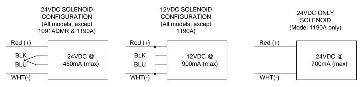
**PR1000 Input Voltage:** 12/24 VDC/VAC (+/-10%) NOTE: 1091ADMR & 1190A will operate at 24VDC only. DC voltage is recommended for optimal performance.
