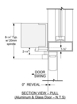
PULL ARM APPLICATIONS: Bottom of operator is mounted 1.5" up from the bottom side of top door frame
