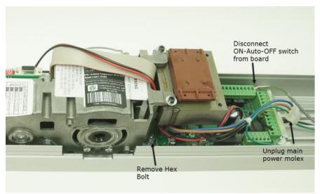
To remove the motor assembly:
