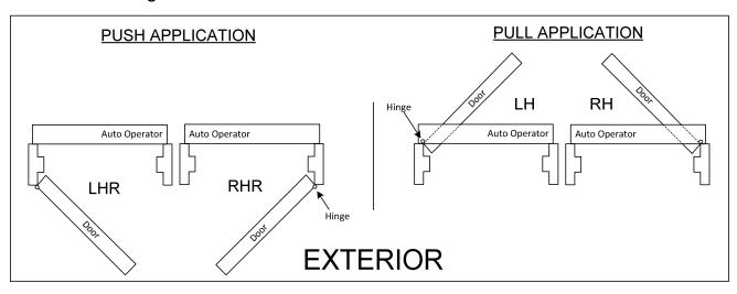
The backplate will mount with the edge nearest the spindle cutout towards to the hinge.
