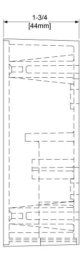
BLACK ABS MATERIAL BOX EQUIPPED FOR WIRED OR WIRELESS APPLICATION. USED WITH 4-1/2" SQ. AND 6" SQ. SWITCHES
