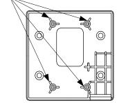
6) Hang the wall switch onto the socket cap screws and tighten down with the allen wrenches provided in the parts bag or with the handle grip allen wrenches. Alternate the tightening of the screws a few turns at a time each from the top to bottom.
