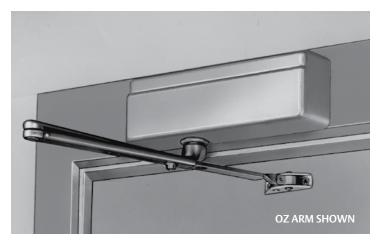
Top Jamb applications - The 351 closer is mounted on the frame face above the door. The foot is mounted on the push side of door. This application is for use on exterior doors opening out to protect the closer from the weather.
