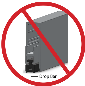
Figure 3 - Improper Drop Bar
