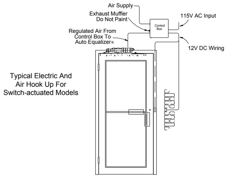
Typical Electric And Air Hook Up For Switch-actuated Models
