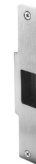
1281 Open back strike for 1 3/4" doors. 8" x 1 1/4" face allow use in mortise lock cutout of stock hollow metal door.
