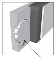
WHEEL STOP INSTALLED - (LOCKS ADJUSTMENT)
