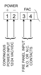
Terminals 1& 2 - Power Input. May be 12 or 24 Volts, AC or DC, uninterrupted. Current requirement is 0.75 Amps for 12 Volts and 0.5 Amps for 24 Volts (check voltage selection jumpers "V" - page 6).
