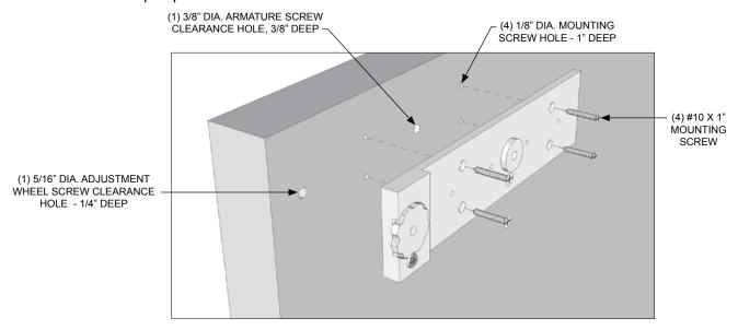
Attach the Armature to the Mounting Plate Assembly using the hardware supplied. Apply the supplied thread locking compound to the threads of the Armature Mounting Screw and firmly tighten with a 3/16" hex wrench. The head of the armature mounting screw must not project beyond the face of the armature. **Failure to properly secure the Armature to the door could result in serious injury or possible security breach.**
