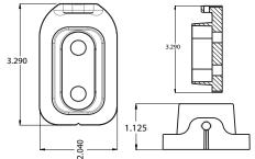
The sill or bottom fitting has a small footprint and, once installed, bottom fasteners are hidden by the mullion tube.
