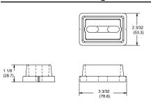
The sill or bottom fitting has a small footprint and, once installed, all fasteners are hidden by the mullion tube.
