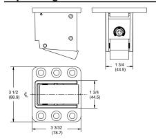
Top fitting has a latch that allows the mullion to be locked back into place without use of the key.
