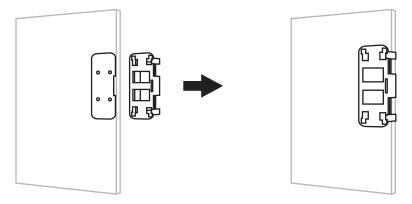
5 Reconnect power supply and install thumbturn side on bracket with the 4 screws removed previously.
