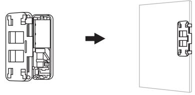
4 Position the 5 screw holes on the mounting bracket with the mounting plate and install screws provided in the box.
