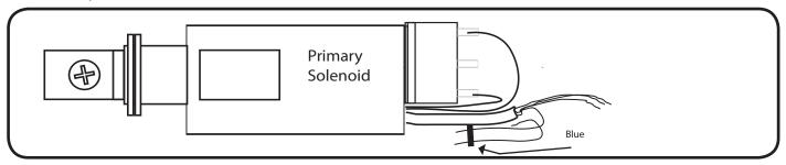
C. Connect White and Red wires from solenoid to White wire from harness. Next, connect Black wire from solenoid to Black wire from harness. Next, connect PM300.
