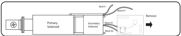
B. Connect Red #1 solenoid wire to White harness wire. Next, connect Black #1 to Black harness wire. Disregard the two Secondary Black wires. Next, connect PM300.
