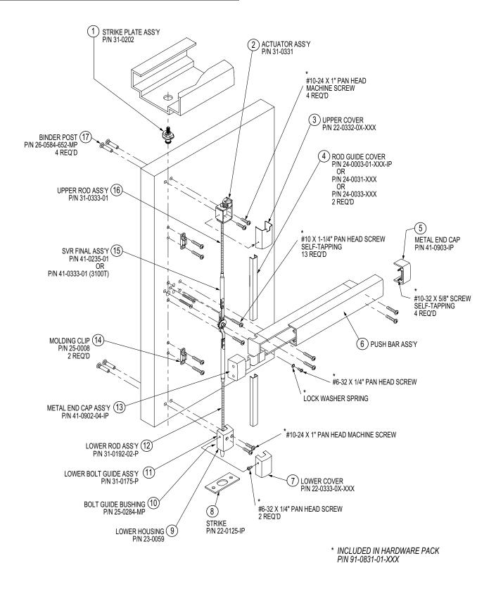
3100 Series Surface Vertical Rod Exit Device (Including 3100T)
