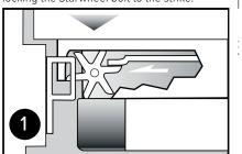
2. When push bar is depressed, the deadlocking slide moves back, allowing the door to unlock from the strike. This unique interlock provides solid security and prevents jamb spreading.
